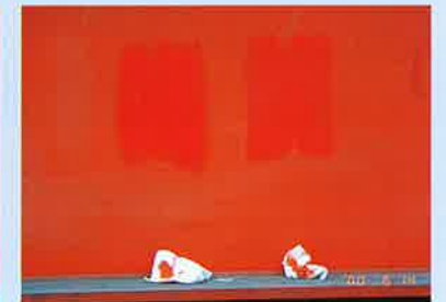
Alkyd part: Chalking and discoloration have occurred
